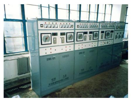
product name: High precision automatic temperature control cabinet Category: Bi-metal Band Saw Units Whole Set Machines -> Heat treatment
